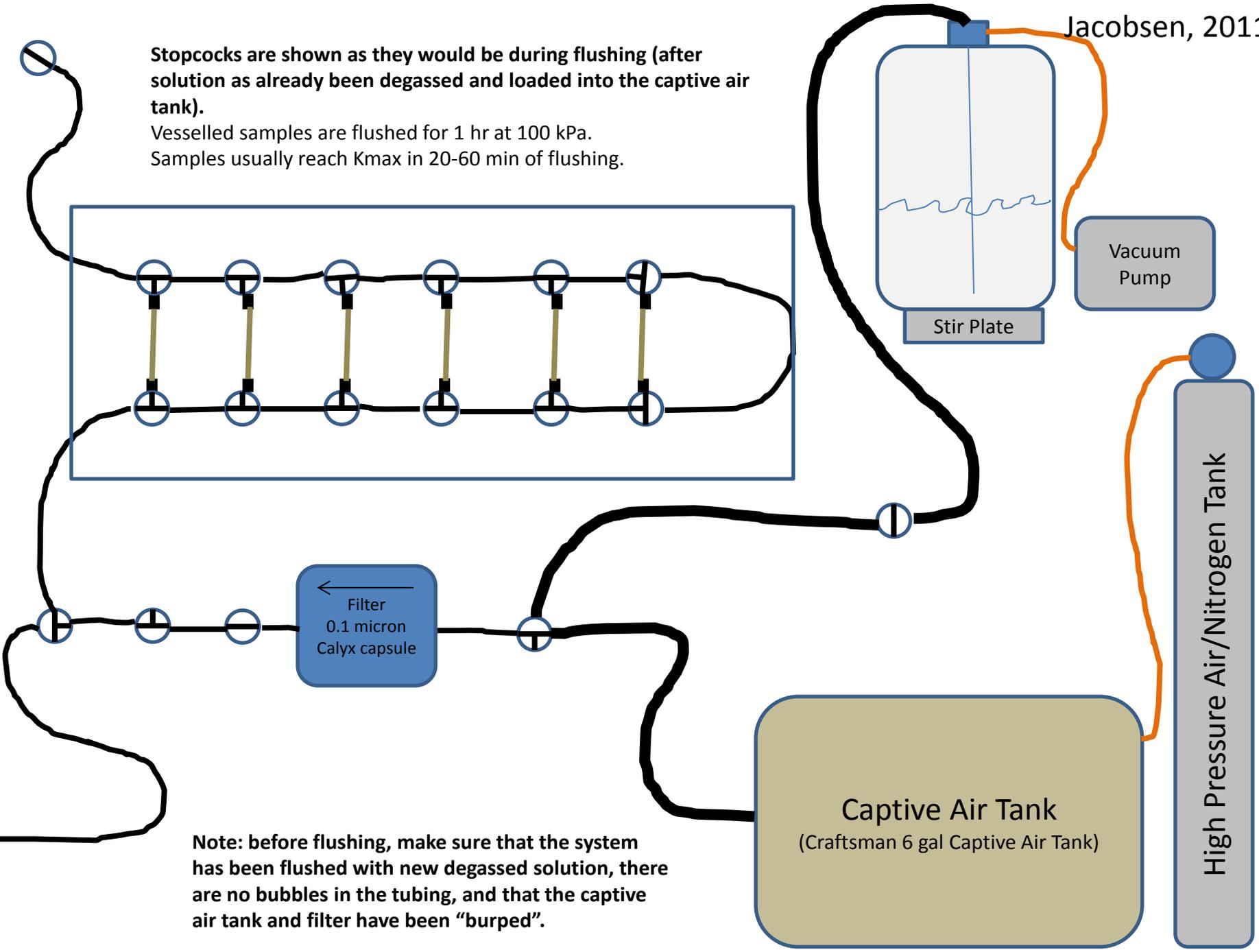
**Note:** before flushing, make sure that the system has been flushed with new degassed solution, there are no bubbles in the tubing, and that the captive air tank and filter have been "burped".
