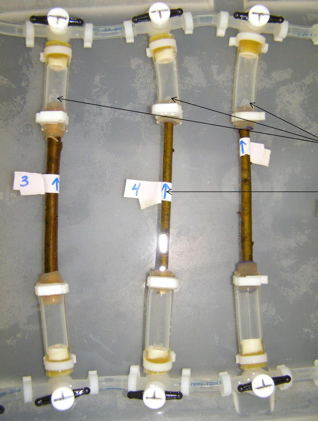
There are no air bubbles in the system when stems are loaded, but bubbles are often visible on the far end of samples during flushing as emboli are pushed out of the xylem.
