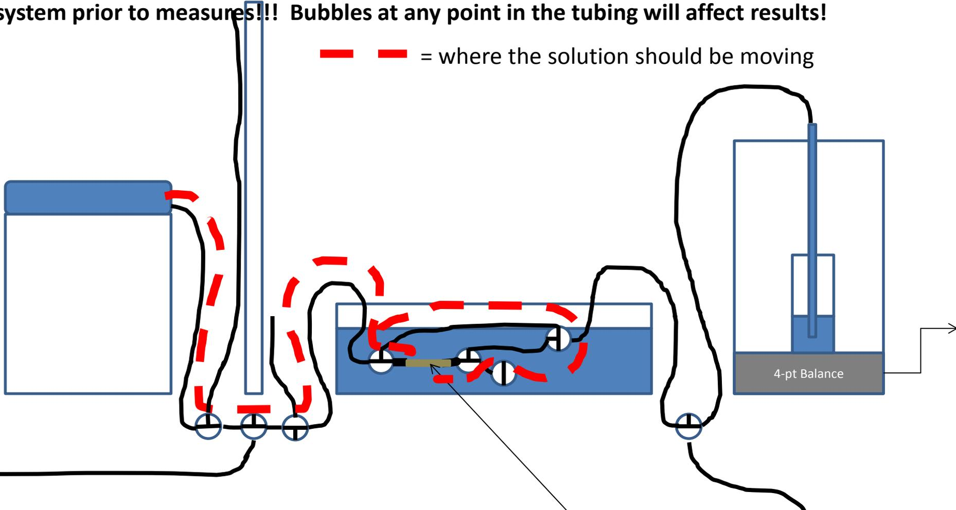
Stem is held in place with latex grommets (latex tubing of many different diameters is cut into small pieces so that samples of any size - usually 6-8 mm in diameter--can be fit into the tubing).
