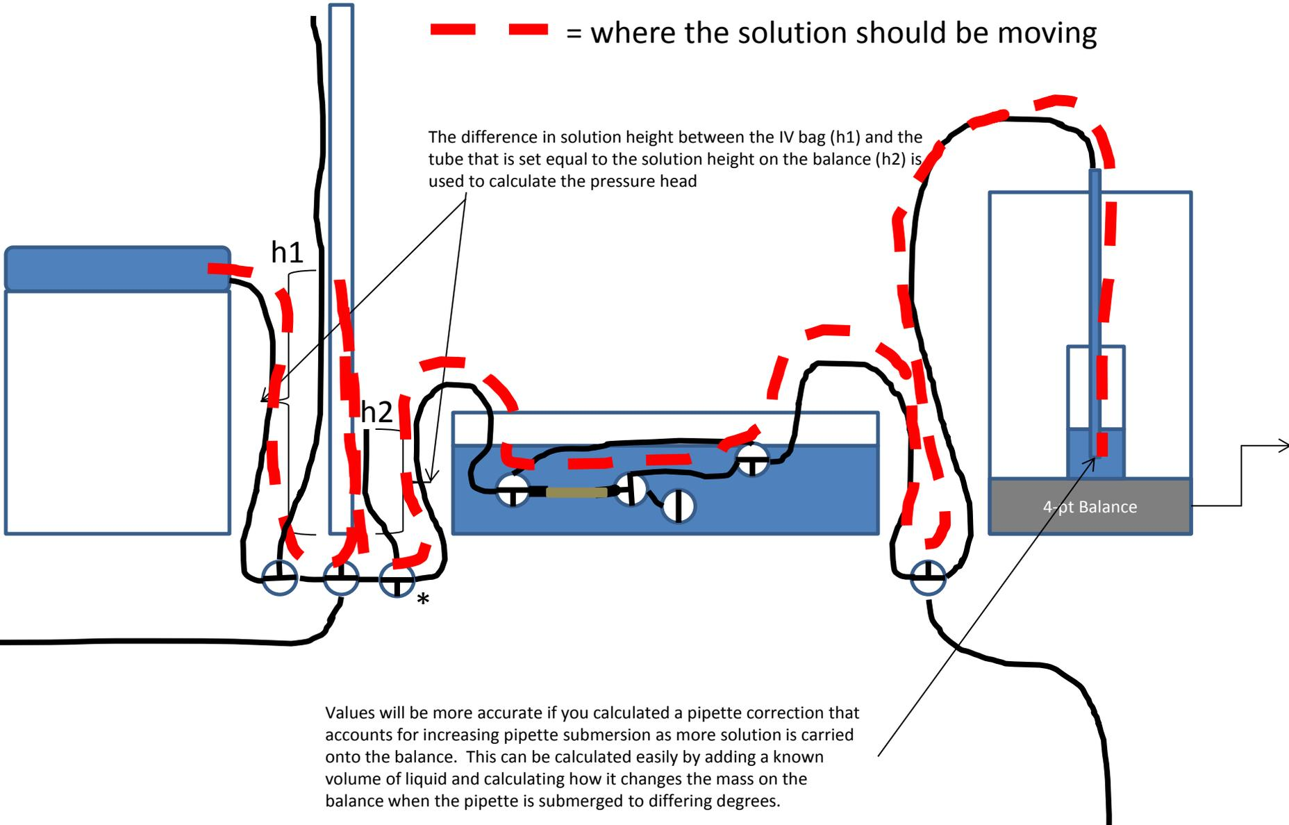
Values will be more accurate if you calculated a pipette correction that accounts for increasing pipette submersion as more solution is carried onto the balance. This can be calculated easily by adding a known volume of liquid and calculating how it changes the mass on the balance when the pipette is submersion to differing degrees.
