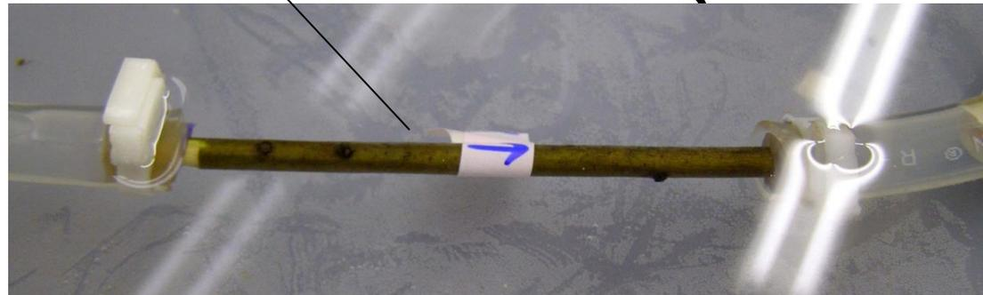
Direction of stopcocks run initial and final (background) flows—these flow measures should be near zero because there is no pressure on the sample. These values tend to become slightly negative in dehydrated stems presumably because the stem parenchyma is taking in solution.
