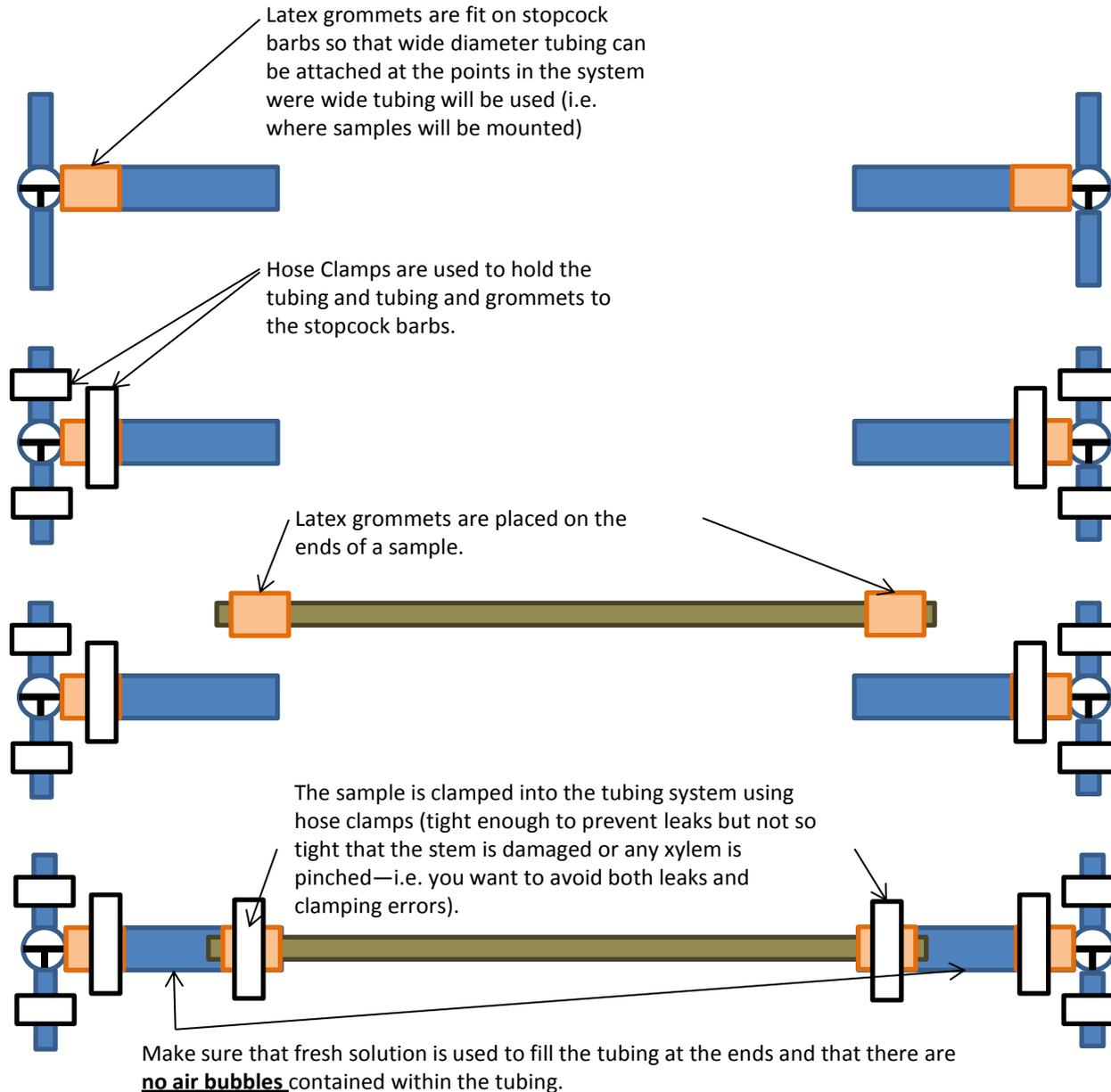
Direction of stopcocks to load a stem—**NOTE: All bubbles must be removed from the tubing system prior to measures!!! Bubbles at any point in the tubing will affect results!**
