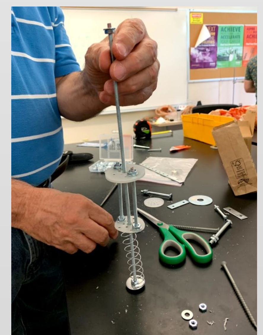
M.R. Fluid Damper Concept
