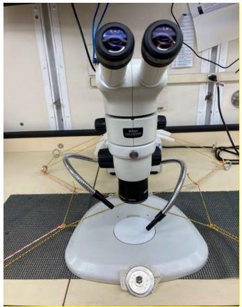
Microscope tied down to keep it from moving with the seas while on board the ship.
