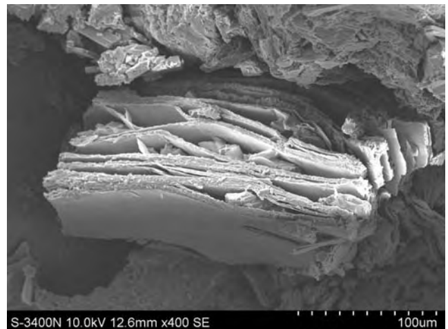
Detrital biotite disrupted by growth of authigenic ankerite along cleavage planes.
