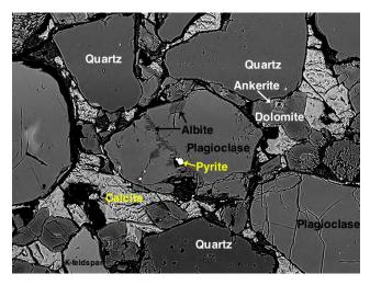
The back-scattered electron imagery obtained using this instrument has revolutionized our ability to study mineralogical and geochemical variations in thin sections. It has also allowed us to make major in-roads into identifying the source of arsenic contamination in groundwater in the San Joaquin Valley.
