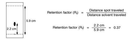
In the example shown above, the spot started at the dotted line on the bottom of the plate. As the solvent moved up the plate, it traveled 5.9 cm but the spot traveled only 2.2 cm. Thus the  $R_{\rm f}$  of the spot is 0.37. Note that the distance the spot traveled is measured from the middle of the spot.
