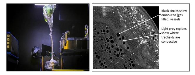
**Figure 3.** The chamber within the microCT that houses specimens. Samples that are up to 50 cm may be put into the chamber and scanned (left panel). Following a reconstruction of a sample, slices of the xylem can be digitally extracted and examined to determine which cells are blocked with gas (black) and which are conductive (light grey) (right panel).
