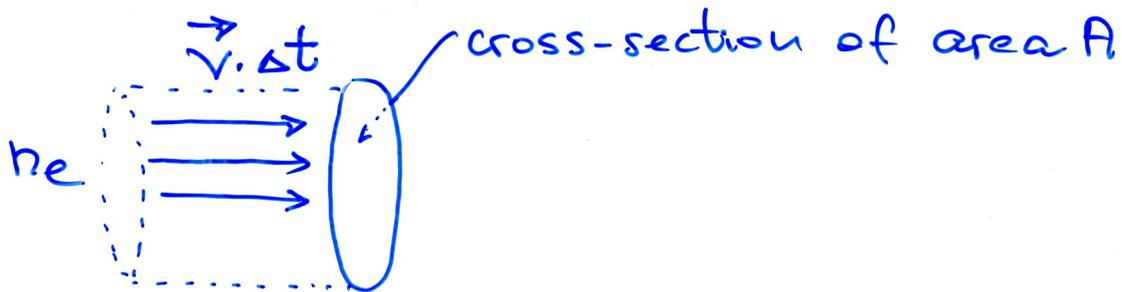
current  $I = \frac{\Delta Q}{\Delta t} = \frac{-e \cdot v_d \Delta t \cdot A \cdot n_e}{\Delta t} = -n_e e v_d A$
