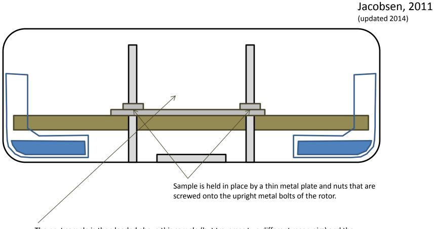
The next sample is then loaded above this sample (but traverses two different reservoirs) and the process is repeated.
