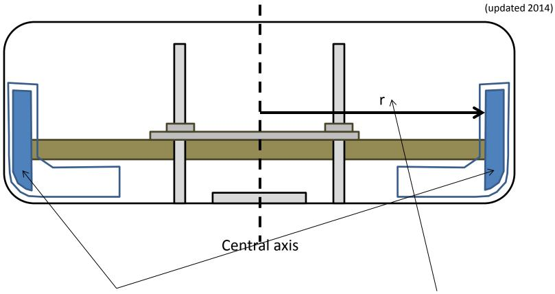
When the rotor is spinning, the solution is held against the vertical walls of the reservoirs and so the ends of the samples under water. Because the same amount of solution is loaded into each reservoir, they balance each other and there is no net flow through the stem while it is spinning.
