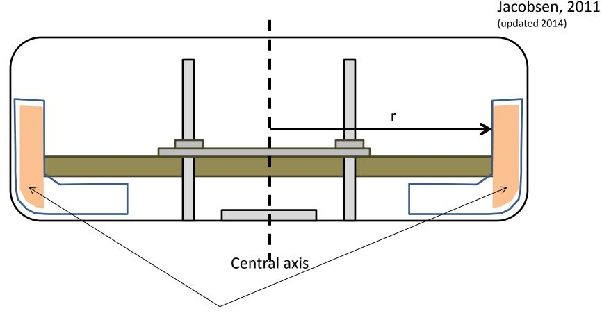
With the hydration reservoirs, the solution is held entirely within sponges both before and after spinning. We fully saturate the sponges with degassed ultrafiltered solution and we have trimmed them so that they reach to the surface of the reservoirs. When using the hydration reservoirs, we keep enough solution in the reservoirs to fill them to their rim when the sponge and solution are present. This makes the calculation of r easier (i.e. from the sample center to the reservoir; see above).
